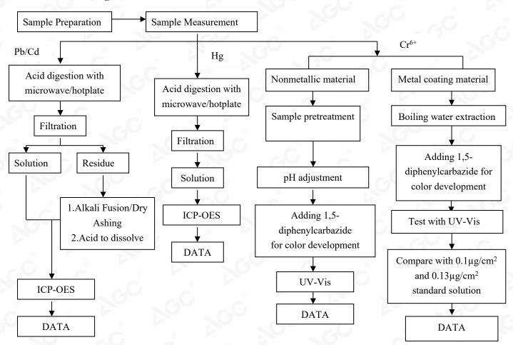
These sample were dissolved totally by pre-conditioning method according to above flow chart (Cr<sup>6+</sup> test method excluded)
